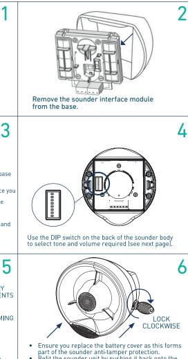
Refit the sounder unit by pushing it back onto the base, push the key all the way in, turn both security fixings back to the locked position on both sides.
